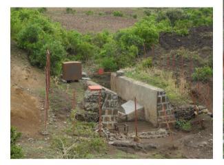
*Photo 15: Hydrological station to measure runoff and sediment transport*
